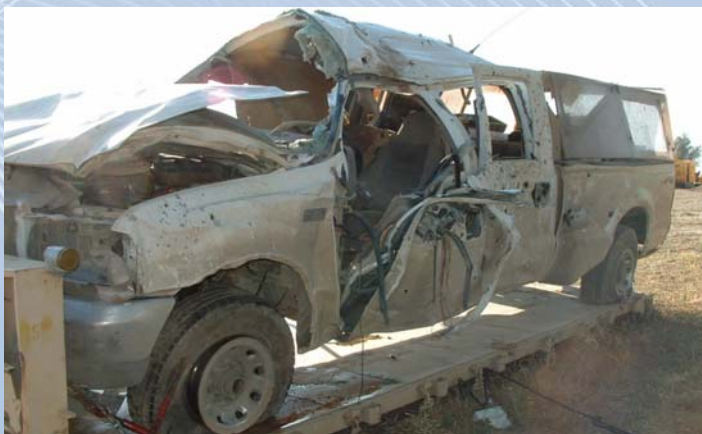
Double cab 4x4 after landmine exploded
