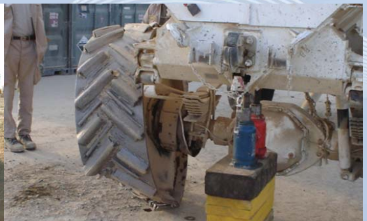
Casspir MkI with fitted Steelwheels after landmine exploded
