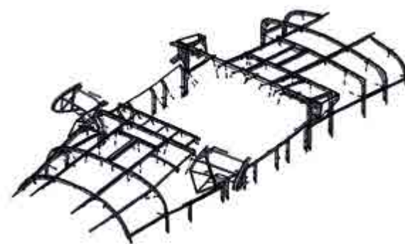
The metallic substructure of the WFF
