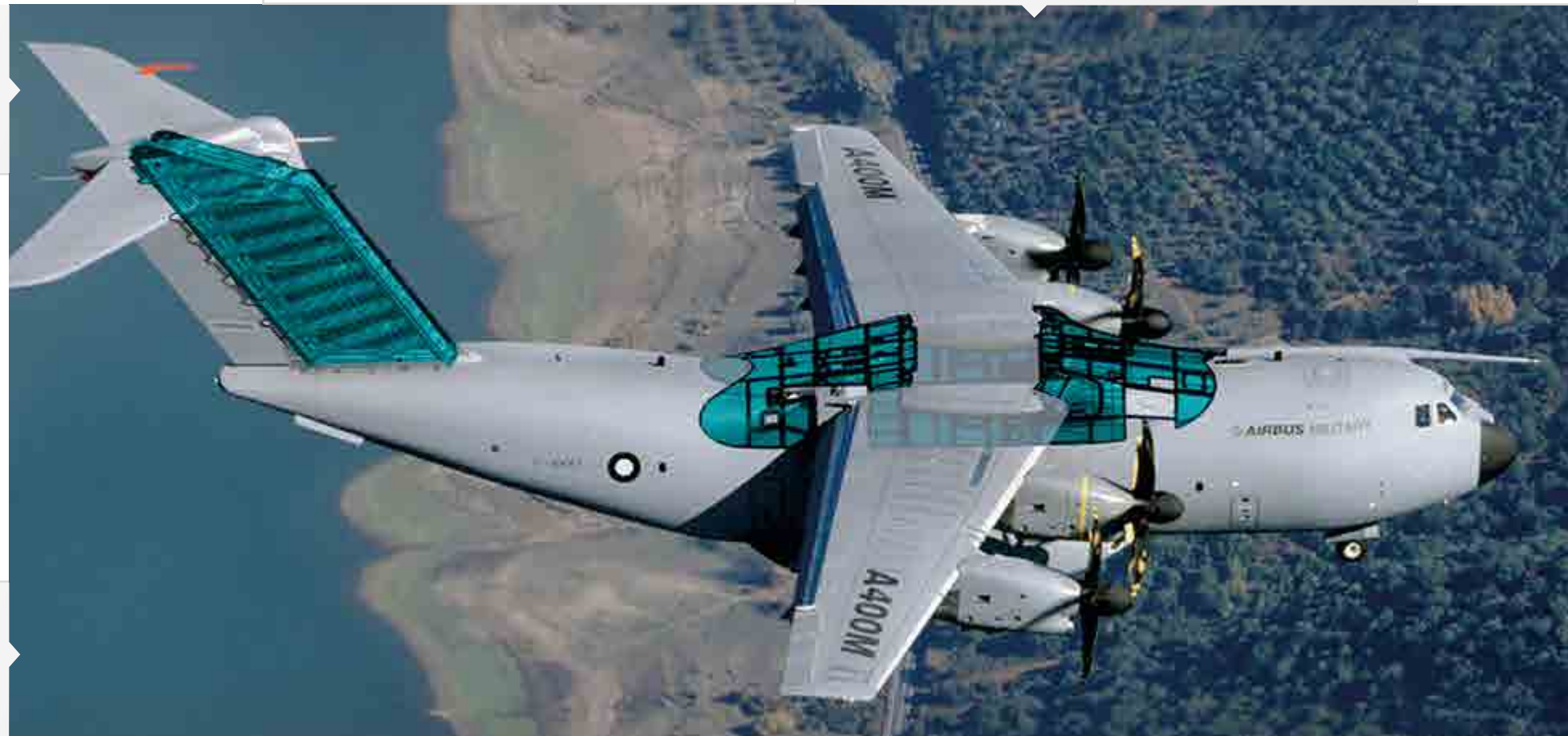
Airbus A400M Top Shell Aft Inner
