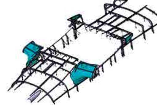
The LH & RH Onglet showing the composite Panels highlighted on the Metallic substructure.
