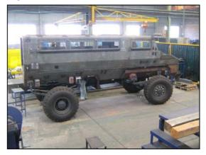
One piece welded and bend single construction V-shaped Mine protected Hull comply to STANAG 4569
