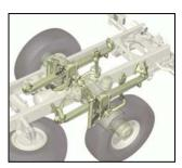
CASSPIR NG2000 is equipped with the well known MB heavy duty axles, built to specifications in Daimler AG and Switzerland. Both axles fitted to CASSPIR NG series are of similar variant as used in the Mercedes Zetros Military Truck of a high axle load carrying capacity. CASSPIR NG2000 is fitted with a 9000 kg load carry capacity axles that allows for potential armour upgrade without vehicle overloading.
