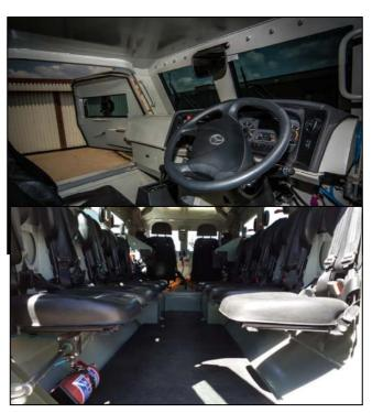
Large open interior with design features to shift the seat configuration as to client requirement. All seats are of the latest and tested ballistic type fitted with a 4 point safety harness system.
