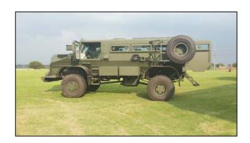
Vehicle is fitted with two crew side doors and one r rear entry exit door. A drinking water tank, two stowage lockable boxes and a battery box are all fitted to the side of the vehicle.
