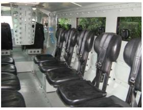
Large open interior with design features to shift the seat configuration as to client requirement. All seats are of the latest and tested ballistic type fitted with a 4 point safety harness system.
