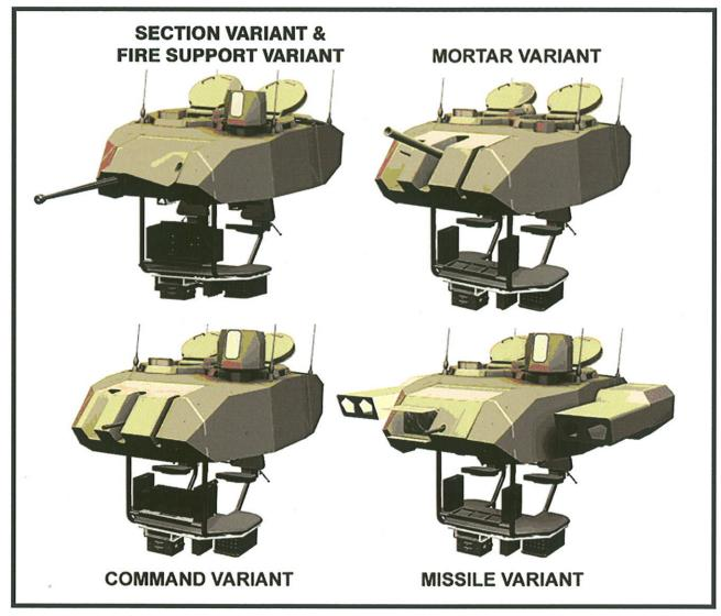
All turrets are designed around the same basic Fighting Compartment Module (FCM) to ensure maximum commonality and re-use of components and modules.
