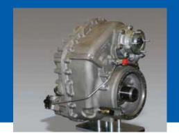
The RGR32MTC transfer case is a light weight, transmission mounted, low noise, helical gear driven customised solution for the RG32M mine hardened armoured patrol vehicles in the 9.5 ton gross vehicle mass range.
