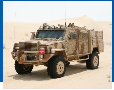
The RG32M LTV is an enhanced mine protected variant of the successful RG32M Patrol Vehicle, that provides even better crew safety and blast survivability.
