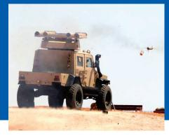
The Missile Stabilised Turret (MST) is a lightweight remote controlled missile stabilised turret, firing the well-known Ingwe anti—tank missile and capable of engaging moving targets from typical 200m to 5 000m, while on the move.
