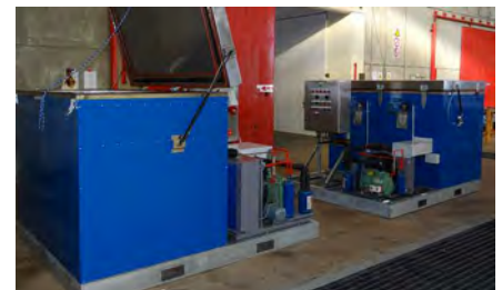
The new cold and hot / ambient units the Test Range obtained to satisfy the requirements of clients, enabling the Range to deliver a more comprehensive service.
