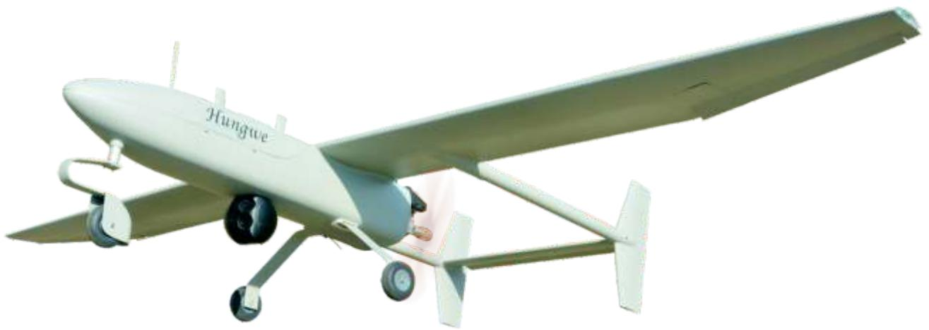
This small UAV has an all-composite, low-drag blended wing design that ensures optimum performance. It is fitted with a day or night payload. The communications link on-board the UAV enables real-time communication up to 100 km from base.
