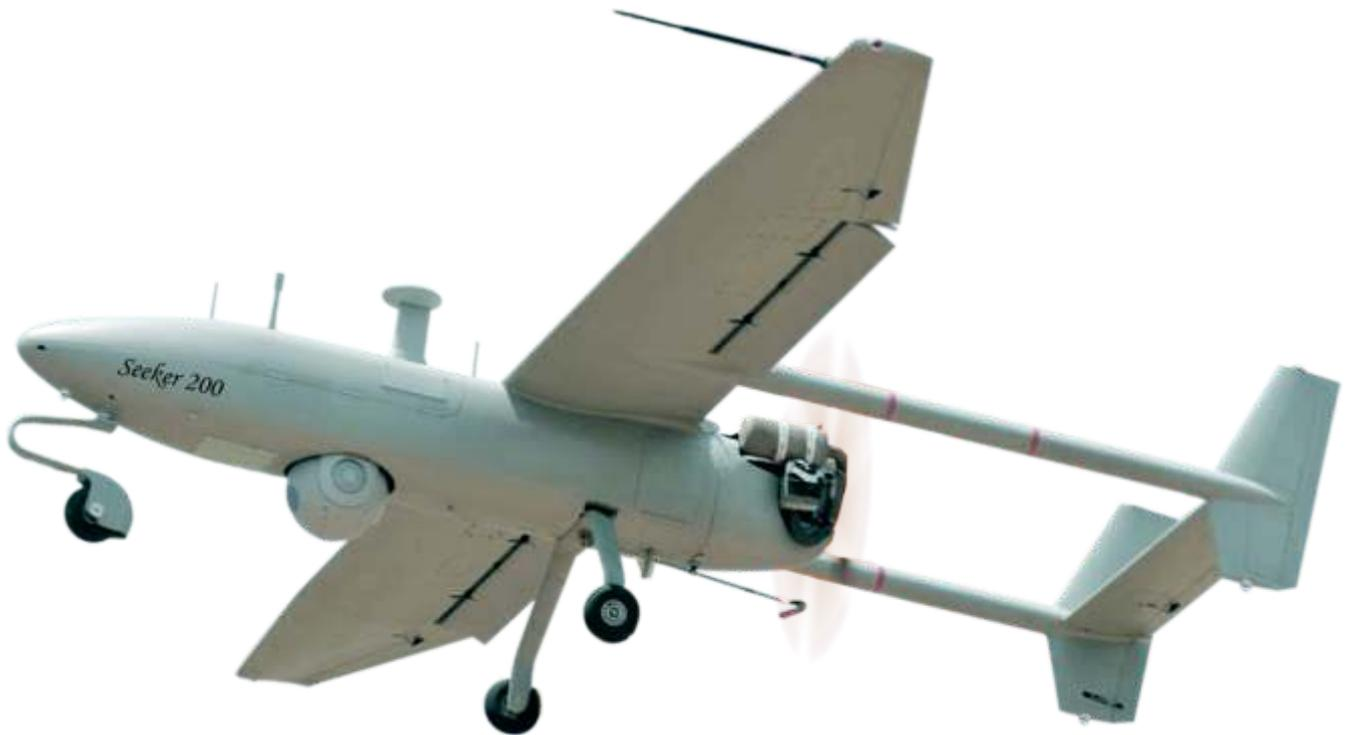
The Seeker 200 tactical Unmanned Aerial System evolved from the battle-proven Seeker II system. This feature-packed derivative offers an engine with long service intervals (> 250 h), long endurance, low noise levels (<70 dB open throttle at 1 000 ft AGL), short take-off distance (~300 m ASL) and a rapid rate of climb (~750 ft/min).
