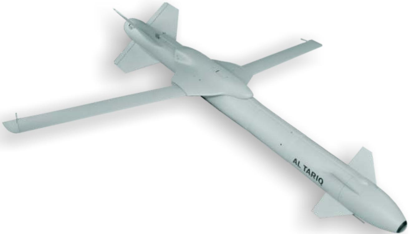
Al Tariq is a family of strap-on bomb kit systems, used on Mk81 and Mk82 bombs. Al Tariq provides the user with all-weather, day or night operational capabilities, utilising GPS/INS guidance or Imaging Infrared (IIR) with complete Automatic Target Recognition (ATR) capability, or a Semi-active Laser (SAL) seeker. The system can also be fitted with an RF proximity fuse for area targeting, using a pre-fragmented warhead. It is autonomous target acquisition with stand-off range.
