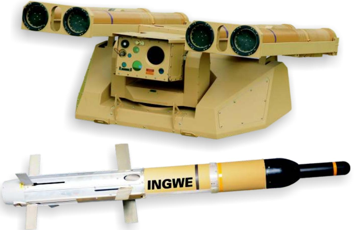
Armed, Long-range, Reconnaissance Turret, ALRRT (Alert) adds to the operational effectiveness of the highly lethal Ingwe anti-armour missile. Available in a variety of configurations (four missiles, two missiles with a 7.62 mm calibre machine gun, etc.), the turret can be integrated on a wide range of vehicles from Light Utility Vehicles (LUV) to heavy Infantry Fighting Vehicle (IFV).
