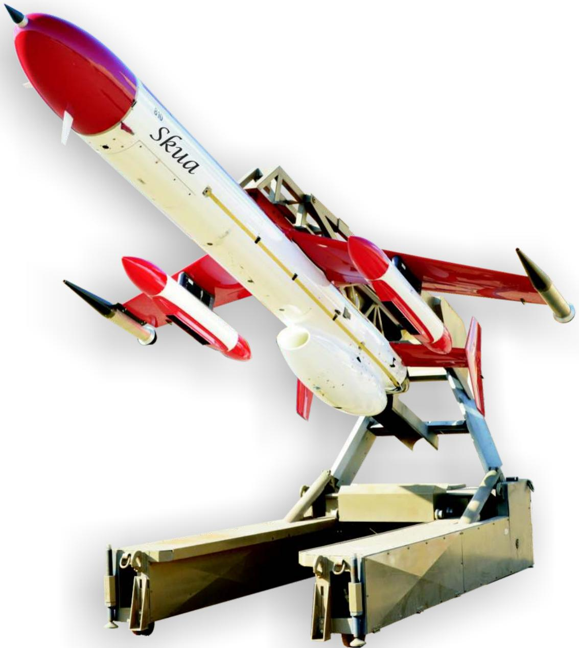
The Skua is a high-speed target drone designed to simulate high-speed attack aircraft during weapon development as well as land, sea and air combat training. The Skua has an all-composite, low-drag airframe with a wingspan of 3.57 m and length of 6 m. Wing hard-points are provided to carry up to 130 kg of tow-targets and signature augmentation equipment. An internal bay can house a payload of up to 30 kg.
