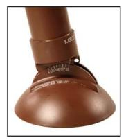
A clamp-on handgrip incorporates a special sight with all data needed. The range, elevation and charge to be used is engraved on the face plate.
