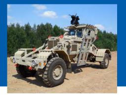
The Self Defence Remotely Operated Weapon (SDROW) is a light-weight weapon system fitted with a Light Machine Gun (LMG) for use on a variety of soft-skinned, Armoured Personnel Carriers (APC) and Mine Protected Vehicles (MPV).
